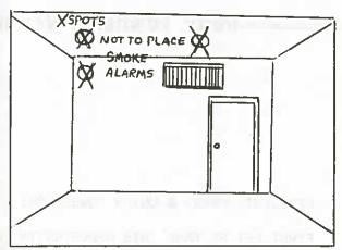
Most detectors are battery operated. The 9 volt battery powered detector is the best. Some are 110 volt wired—in electric detectors. The battery type is the best in most cases because it can be mounted at the best spot by merely attaching it to the ceiling where you need it.
